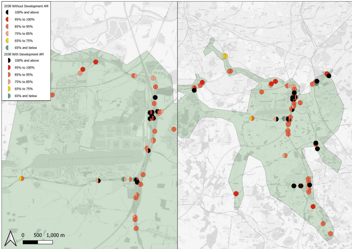
Figure 3.15: Forecast Node Volume-Capacity Ratio for 2038 Core and 2038 With Development
