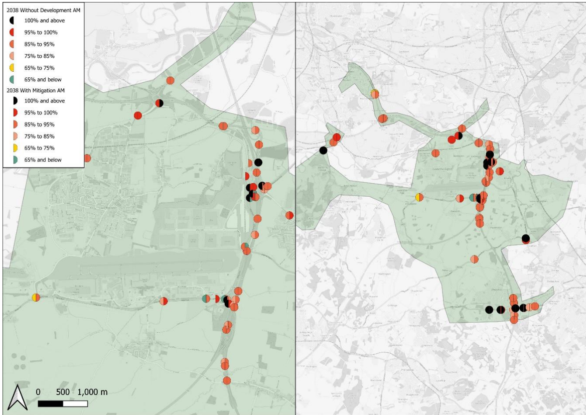
Figure 4.15: Forecast Node Volume-Capacity Ratio for 2038 Core and 2038 With Mitigation
