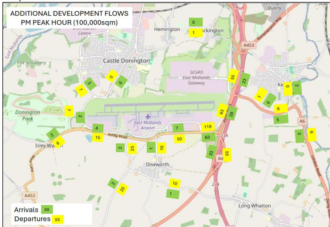
Figure 2: Traffic Assignment of 100,000sqm GFA Mezzanine Floorspace (evening peak hour)
